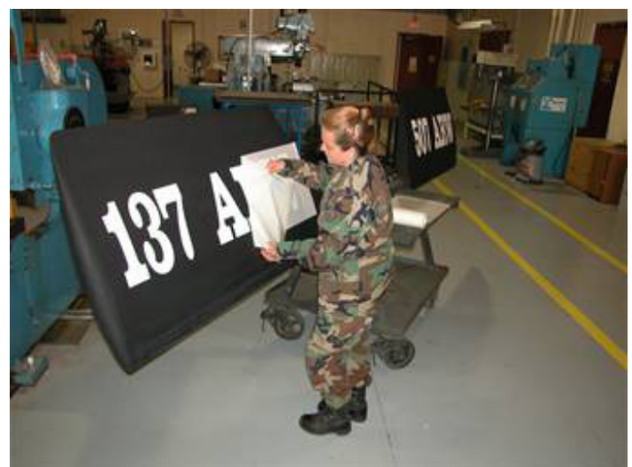
Staff Sgt. Sue Hathaway, a structural repair and corrosion control technician with the Air Force Reserve's 507th Air Refueling Wing, peels away transfer paper backing while applying new lettering to a KC-135 ruddervator.
